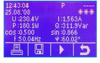
Energy meter testing on site – functions of computing meter error directly
