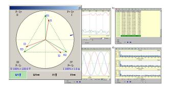
Energy meter testing on site – functions of computing meter error directly in percentages with method of setting time of measurements or number of impulses and functions for verification of energy meter counters. Input in S0 standard is used for testing energy meters with impulse output. Miniature photo head CF101 is used for automatic counting of meter rotor turns for testing Ferrari meters.
