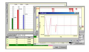
Recording and analyzing of power quality according to the EN50160.
